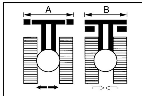
The setting of the track width is with the control lever for extendable track width (1).
