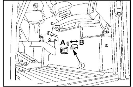
The air is guided to the air nozzles (1) via the heat exchanger.
