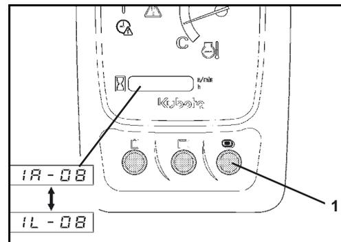
After setting the flow rate for the operating mode selected, you can either switch to the next operating mode or exit the settings screen.
