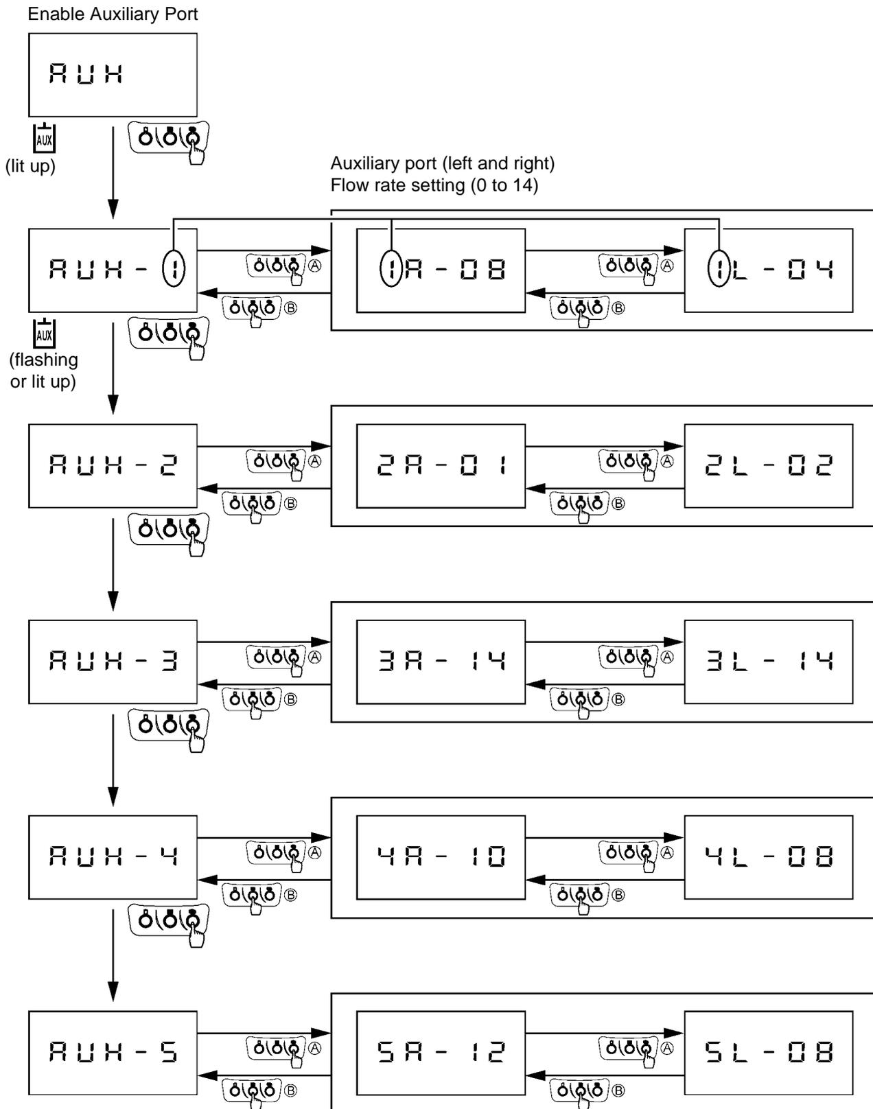
(A) Press and hold the display selector switch.
