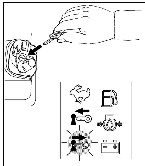
8. Turn key into position RUN to complete the registration process.
