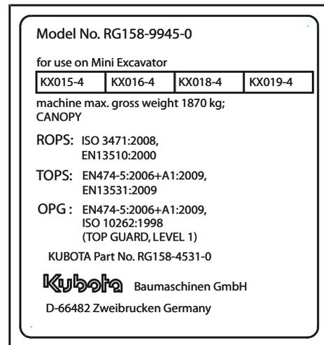
Use utmost care to avoid any risk of tipping, slipping, or other potential risks implied when lifting loads. The operator must
