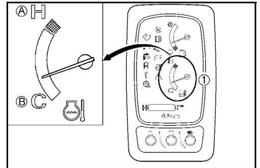
When the machine is being operated at or close to full capacity, the temperature of the coolant can rise a little higher than normal. The indicator Coolant temperature (1) blinks and the message appears in the display as shown in the figure on the right.
