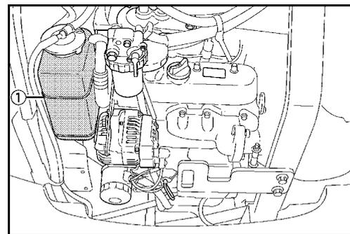
If the coolant expansion reservoir was completely empty, check the coolant level in the radiator.
