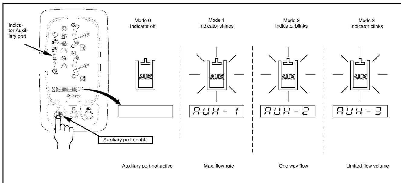
If the auxiliary port is switched on and a mode of operation has been selected, the set flow rate in the right auxiliary port connector and then in the left auxiliary port connector is indicated for few seconds in the display (2) by pressing the display selector switch (1).
