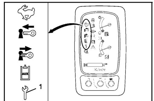
If the maintenance interval indicator has to be replaced because of a defect, the meter is set back to "0". Ask your KUBOTA dealer about this.
