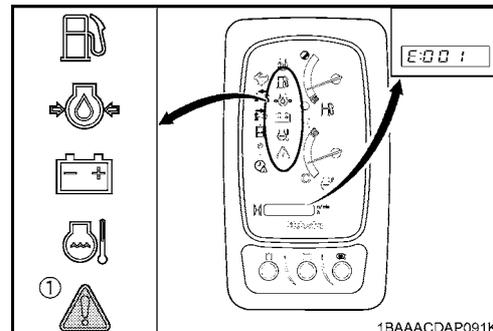
If the engine oil pressure becomes too low during operation, the engine must be stopped immediately. The engine oil pressure indicator (1) lights up, the warning light (2) flashes red and the display message as in the figure on the right appears.
