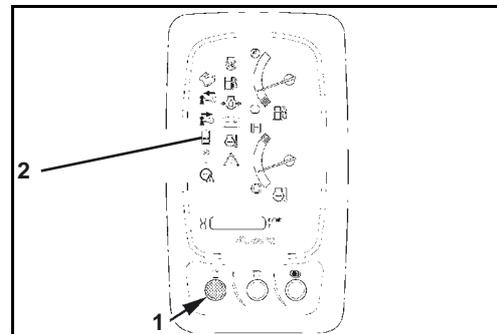
The set flow rate in the right auxiliary port connector and then in the left auxiliary port connector is indicated for few seconds in the display by pressing the display selector switch (1).
