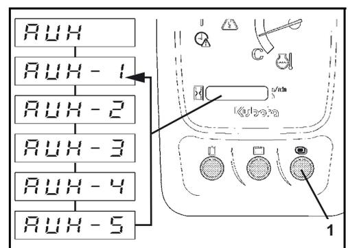
When the selected flow rate is shown on the display, you can use the display selector switch (1) and the menu button (2) to increase or decrease the flow rate.
