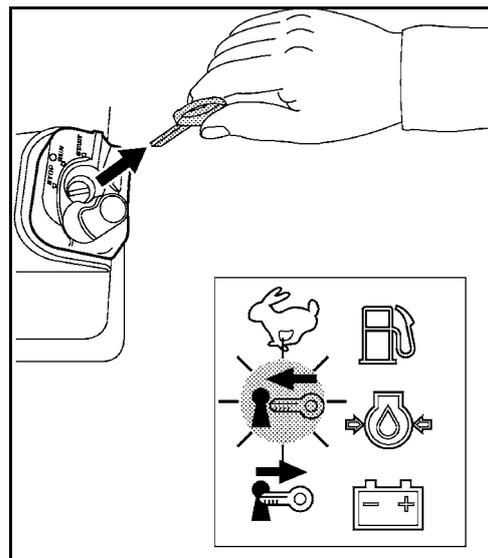
7. After a short moment, the indicator Pull out key blinks. This points out the fact that the black key has been registered for this vehicle.
