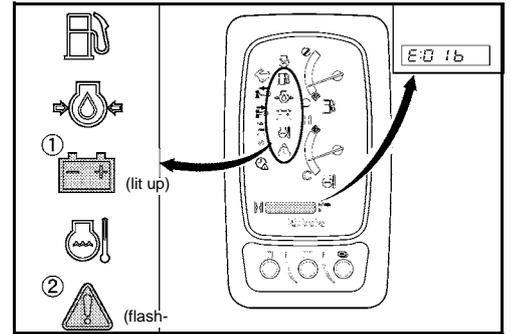
The needle of the coolant temperature gauge (1) should be in the area between "C" (COOL) and "H" (WARM). If the needle rises up to range "H" (Red), cool down the engine by changing into idle.
