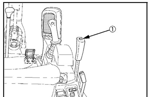
A tone sounds and the indicator (1) shines. Renewed operating of the push button travel speed switches back to normal speed. Besides, audible signal sounds and the indicator goes out.
